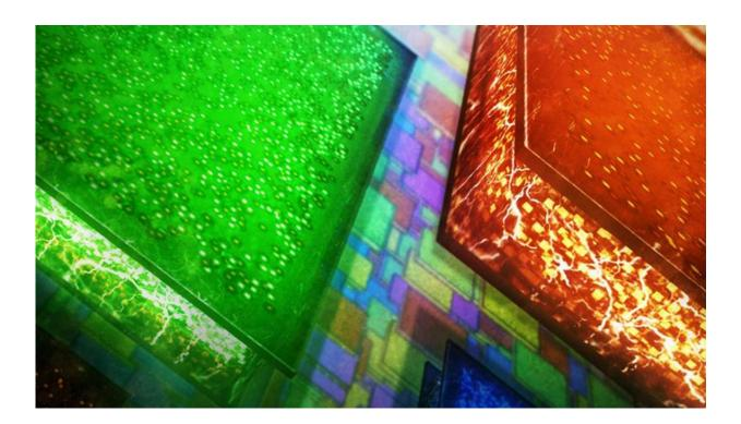
Dynamic color tunability of amorphous photonic structures in response to external electrical stimuli using electrophoretic deposition process. Credit: Ryan Chen/LLNL
