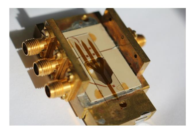
The brass block serves as an electric ground plate ensuring an efficient insertion of the RF currents to the antennae and, on the other hand, microwave connectors mounted to the block allow for the embedding of the device into our microwave setup. Credit: Fischer/Kewenig/Meyer
