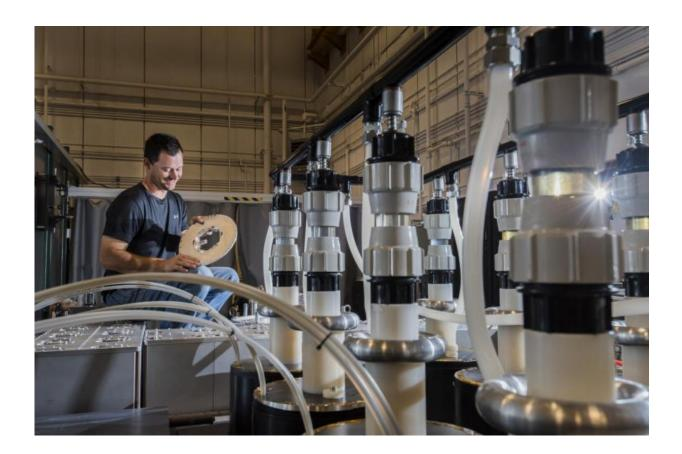
Sandia National Laboratories technologist Joshua Usher loads a target into the main power flow section of Veloce, a Sandia pulsed-power generator. The machine uses pressure rather than chemicals to form nanocomponents from nanoparticles. Credit: Randy Montoya
