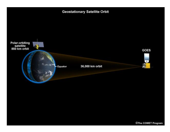
Geostationary satellites like Geo-Carb and the GOES weather satellites (shown here) are positioned over the equator at an altitude of about 36,000 km (or 22,300 miles) above Earth's surface and orbit at the same speed as the Earth's rotation, making them appear to stand still. OCO-2, like the Low Earth satellite shown here, samples a much narrower area. Credit: UCAR
