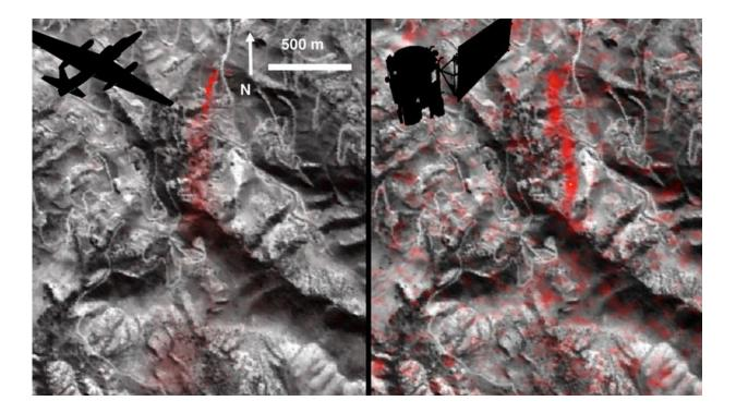
These images of the Aliso Canyon, California methane leak, taken 11 days apart in January 2016, are the first time the methane plume from a single facility has been observed from space. Photos were taken by instruments on (left) a NASA ER-2 aircraft at 4.1 miles (6.6 kilometers) altitude, and (right) NASA's Earth Observing-1 satellite in low-Earth orbit. Future instruments will provide more precise measurements. Credit: NASA
