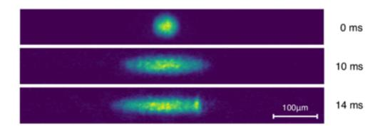
Experimental TOF images of the effectively 1D expanding SOC BEC for expansion times of 0, 10, and 14 ms.
