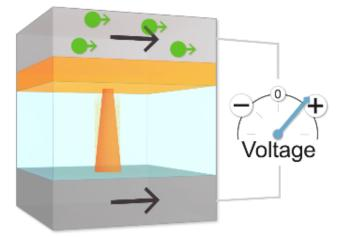
When a bias voltage is applied, copper diffuses through the oxide, forming a low-resistance channel.
