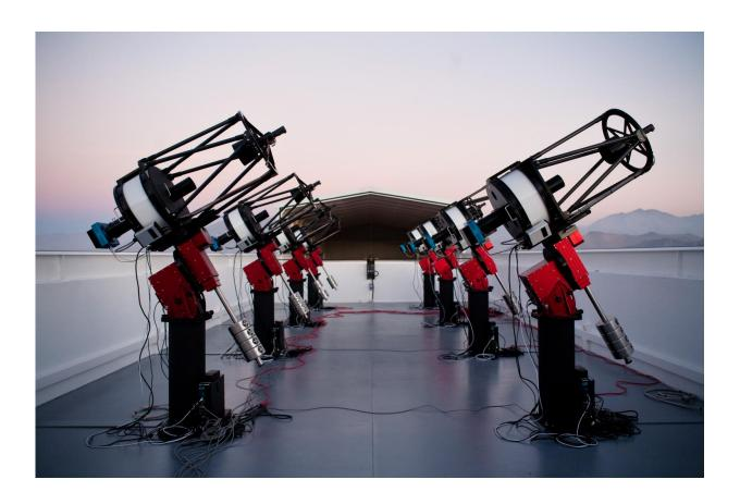
The MEarth-South telescope array, located on Cerro Tololo in Chile, searches for planets by monitoring the brightness of nearby, small stars. This photograph shows the array, comprising eight 40-cm telescopes, at twilight. Credit: Jonathan Irwin
