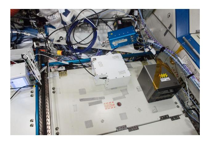
Seen center of the image, the Fast Neutron Spectrometer will help accurately detect neutrons in space. The neutrons are potentially harmful to humans. Credit: NASA
