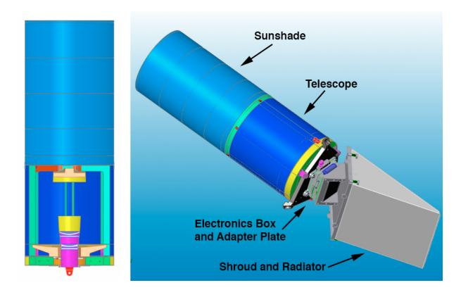
The ShadowCam instrument will acquire images of shadowed regions of the moon using a high-resolution camera, telescope, and highly sensitive sensors.
