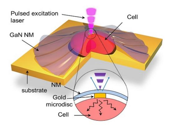
The gallium nitride nanomembrane (GaN NM) is shown attached to a cell. When a pulsed laser is directed onto the nanomembrane, heat is transferred to the cell via a gold microdisc. By monitoring the emitted photoluminescent light (blue arrows), the researchers can calculate the thermal transport properties of the cell. Credit: KAUST Rami ElAfandy
