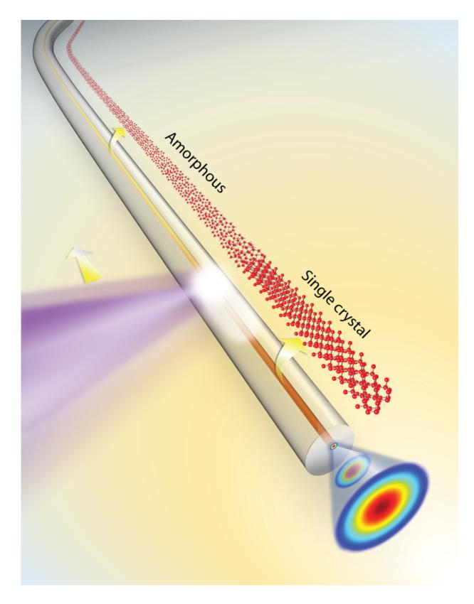
Amorphous silicon core inside a 1.7-micron inner-diameter glass capillary.
