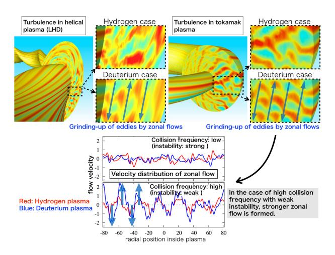
Comparison of turbulence in helical LHD plasma (left) and in tokamak plasma (right). In the red color area, strong eddies and waves are generated. In a deuterium plasma with large ion mass, the zonal flows are grinding eddies and waves into small sizes and suppressing turbulence. The zonal flow is formed
