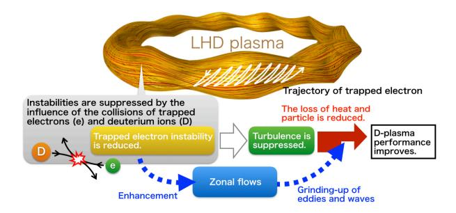
A schematic image of trapped electron instability and the mechanism for the suppression of turbulence in deuterium plasma. When ion mass is larger, instabilities are reduced and the zonal flow increases, and the loss of heat and particles in the plasma is suppressed. Credit: Dr. Motoki Nakata
