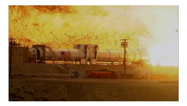
Testing the Space Launch System—NASA's most powerful rocket is designed to carry the Orion deep-space capsule
