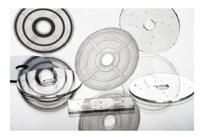
Microfluidic devices for performing various assays were created with the tools in Lincoln Laboratory's Technology Office Innovation Laboratory. Credit: Nicole Fandel
