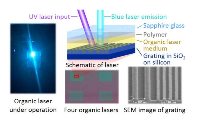
Photograph of a blue organic thin-film laser under operation along with microscope images and a schematic of the lasers. By optimizing the device structure and using appropriate materials, the duration of lasing was extended up to 30 ms, which is more than 100 times longer than previously possible. The schematic is a generalized representation of the structure and is not to scale. Credit: Atula S. D. Sandanayaka and Willam J. Potscavage, Jr.
