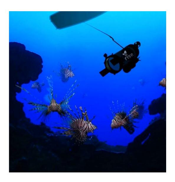
In this artist rendering provided by Robots in Service of the Environment, a new robot that hunts the dangerous and invasive lionfish made its debut in Bermuda in April. It stuns lionfish with an electric current and then the fish is vacuumed
