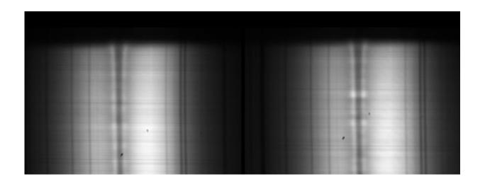
A first-light image from CryoNIRSP. It delivers two spectra simultaneously with opposite polarizations (the left and right panels above). This image shows light from near the edge of the Sun spread out horizontally in wavelength, near the wavelength of a prominent absorption line of Calcium. Credit: UH Institute for Astronomy
