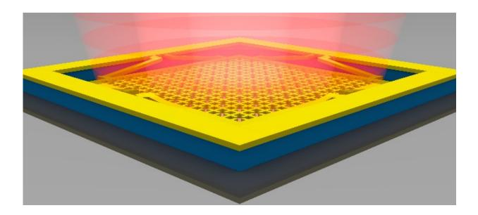
Room temperature MEMS metamaterial, which can achieve reconfigurable infrared intensities equivalent to a temperature change of nearly 20 degrees Celsius. Credit: Xinyu Liu, Duke University
