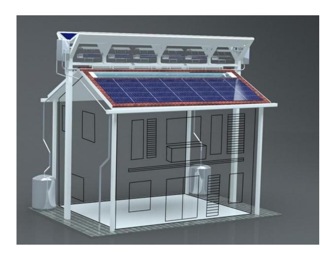
The v-shaped structure on the roof guides wind into a series of turbines to generate energy. Solar cells are washed by a rainwater cooling and cleaning system. Credit: University of Malaya
