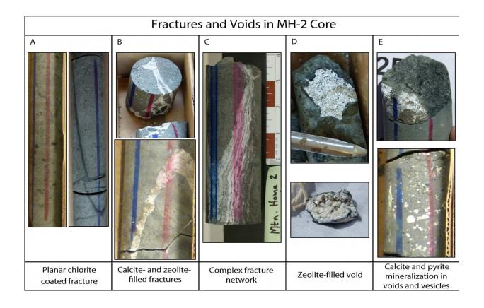
Examples of fractures and vesicles in the MH-2 core. Credit: J.A. Kessler, The Geological Society of America, and Lithosphere
