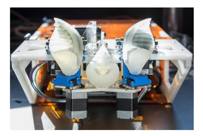
This robotic sonar head mimics the emission and reception dynamics of the horseshoe bat, which uses small movements of the ears and noseleaf to encode extra information in sonar pulses. Credit: Logan Wallace/Virginia Tech
