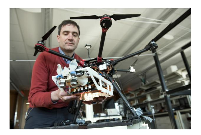
Virginia Tech associate professor Rolf Mueller has discovered that small movements of horseshoe bats' ears and noses help them navigate in complex natural environments. This research has led to the design of a bat-inspired robotic sonar head, shown here being attached to a drone, with a movable 'noseleaf' and 'ears.' Credit: Logan Wallace/Virginia Tech
