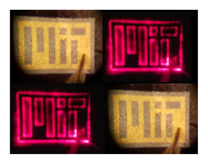
This image shows LEDs grown on graphene and then peeled.
