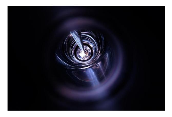
Preparation of the GERDA experiment: Lowering the germanium detector array into the liquid argon tank - view from top.
