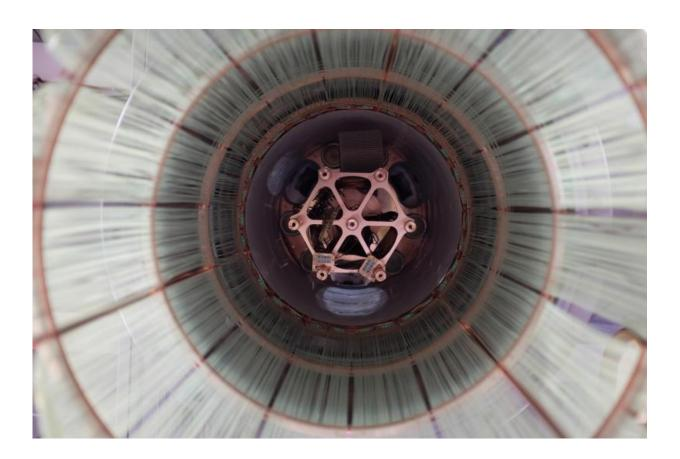
View from bottom into the GERDA experiment: The fiber shroud of the liquid argon veto and the copper. Credit: V. Wagner/GERDA collaboration
