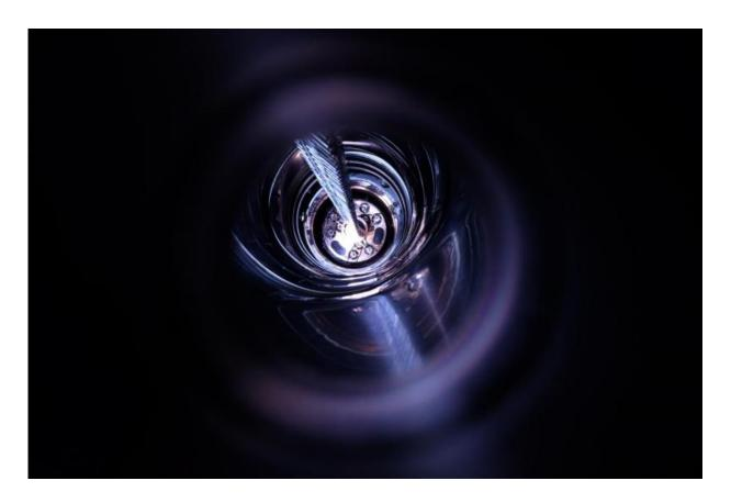
Preparation of the GERDA experiment: Lowering the germanium detector array into the liquid argon tank - view from top.
