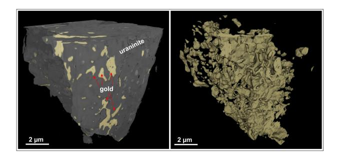
The left picture shows uraninite (uranium ore) that surrounds gold. In the right picture, a computer programme was used the remove the uraninite to illustrate the large volume hidden in the uranium ore. Credit: S. Fuchs, GEOMAR.
