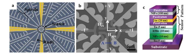
a. Schematic representation of the sensor-integrated magnetic spider web; b. Scanning electron microscope (SEM) image of the sensor integrated with the
