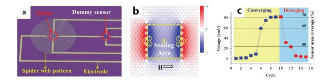
a. A photo of the magnetic spider web chip integrated with the magnetoresistive sensor; b. Landscape of effective stray field depending on the particle location with respect to sensing area of the sensor; c. The measured sensor signal. Credit: DGIST
