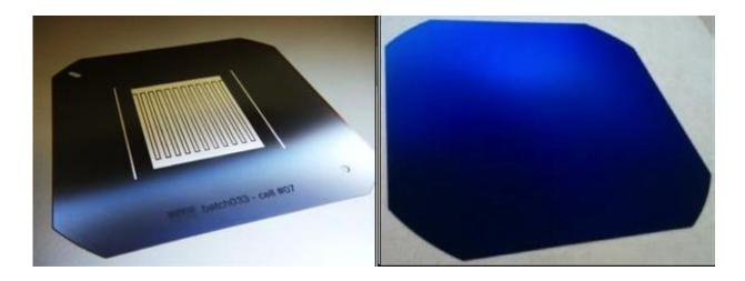
Back of the solar cell, with positive and negative electrical contact. Front of the cell with no shadowing. Credit: Ecole Polytechnique Federale de Lausanne
