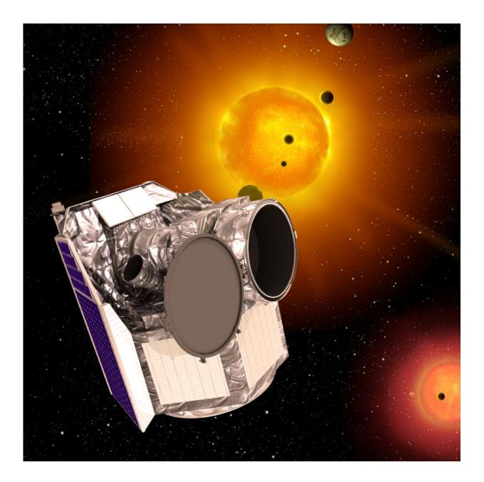
Cheops is a small space telescope dedicated to observing nearby stars that are already known to have planets. Through very precise measurements of the slight dimming of the stars as the planets pass in front of them, astronomers will be able to determine the sizes of the planets and learn more about how planetary systems form. The satellite is being built as a collaboration between ESA and a
