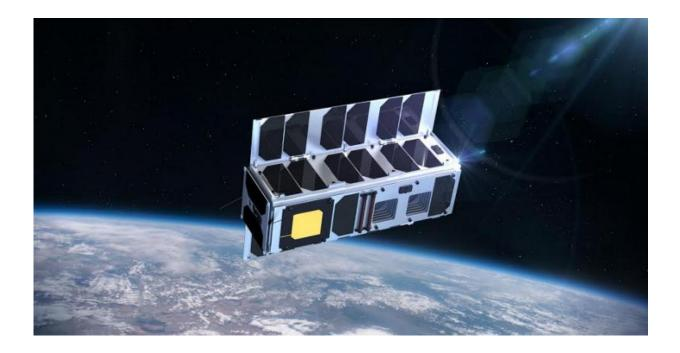
Estonia plans to launch a CubeSat into space in early 2019 aiming to test advanced technologies, including a plasma brake for deorbiting satellites and electric sail propulsion. The mission, named ESTCube-2, will serve as a prototype of Estonia's future moon-orbiting spacecraft.
