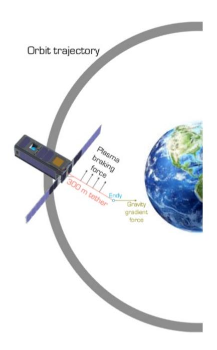
Schematics of plasma brake experiment. Credit: Iakubivskyi et al., 2017/Tartu Observatory
