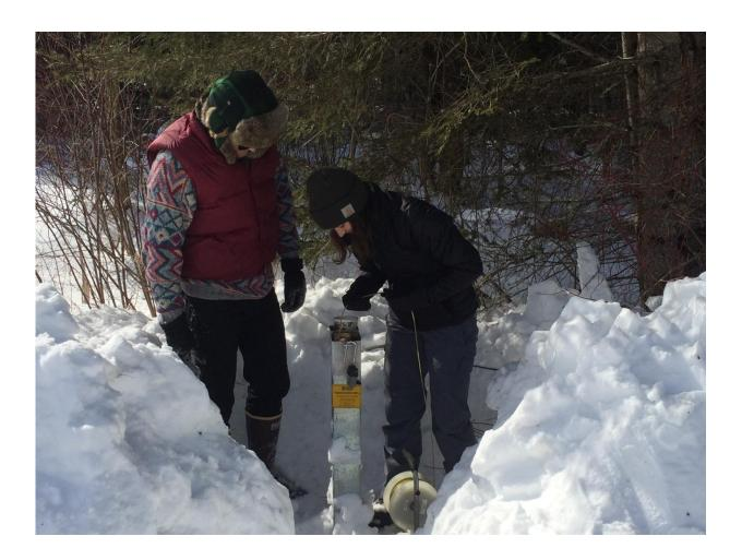
At left, Seth Oliver with Leah Santangelo, right, both hydrogeology UMass Amherst graduates, taking water level measurements at a till site in Blandford, Mass., for a recent study of natural groundwater storage reservoirs in New England by hydrologist David Boutt at the University of Massachusetts Amherst. For the first time, they quantified upland aquifer systems dominated by thin deposits of surface till -- a jumbled, unsorted material deposited by glaciers,
