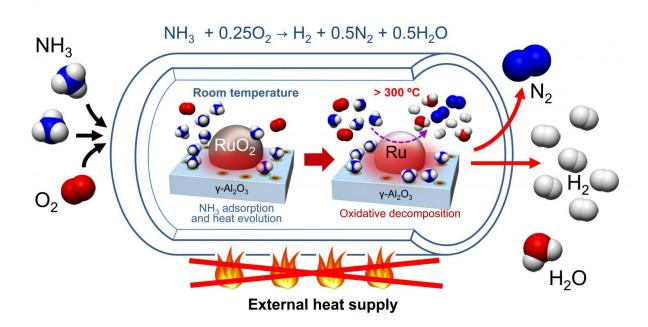
H2 production from ammonia and oxygen triggered at room temperature without external heat input. Credit: Oita University
