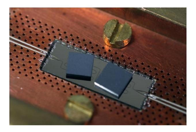
Two black diamonds on a superconducting chip (12x4mm). The wiggly line is a resonator, coupling the two diamonds.
