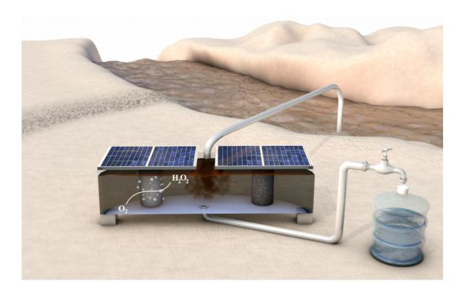
Schematic illustration of an on-site water purification system for rural communities. Powered by solar panels, the low-cost, portable device produces hydrogen peroxide from oxygen gas and water. Credit: Zhihua Chen/Stanford University
