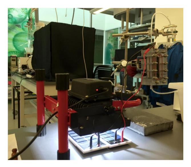
Sized to fit in one hand, this portable, low-cost device uses oxygen gas and water to produce hydrogen peroxide, which can be used to purify water in rural communities. Credit: Zhihua Chen/Stanford University
