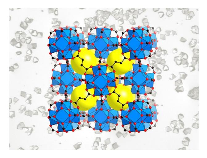
A schematic of a metal-organic framework. The lines in the models are organic linkers, and the intersections are multi-metallic units. These are building blocks that Omar Yaghi stitches together into crystalline sponges using new reticular chemistry. The yellow balls represent the porous spaces that can fill up with water. The background image shows the many cyrstals of MOF that are combined in the water harvester. Credit: UC Berkeley and Berkeley Lab
