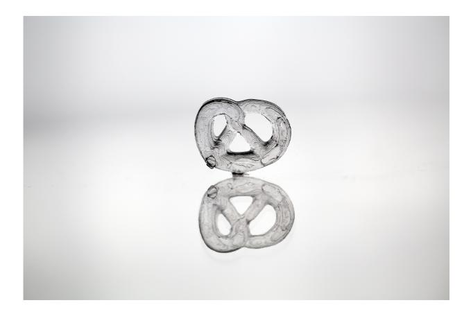
A three-dimensional pretzel generated by three-dimensional printing in fused silica glass. Credit: NeptunLab/KIT
