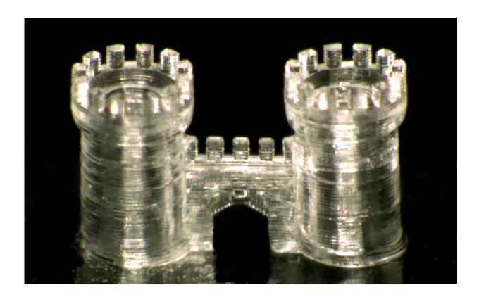
A three-dimensional structure of a castle gate printed in fused silica glass. Credit: NeptunLab/KIT
