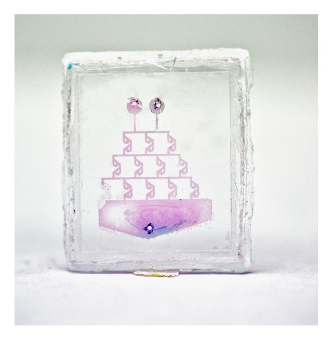
A microfluidic Tesla mixer cascade chip generated by three-dimensional printing in fused silica glass. Credit: NeptunLab/KIT
