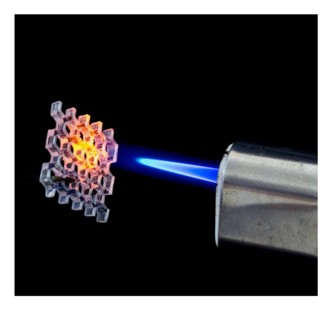
Honeycomb structure printed in fused silica glass exposed to a flame of 800 °C showing the high thermal shock resistance of the printed glass part. Credit: NeptunLab/KIT
