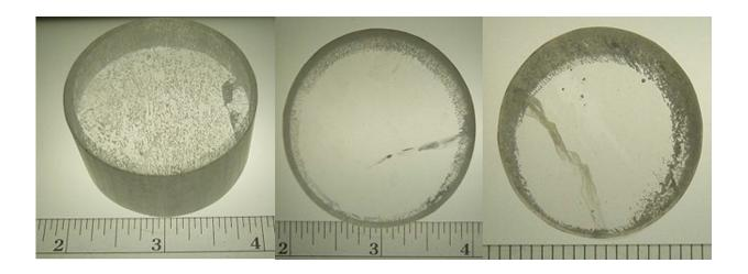
CLYC crystals grown in on Earth often contain imperfections such as inclusions (left), cracks (middle) and grain boundaries (right). The goal is to understand their formation without the interference of convection to improve crystal growth on Earth. Credit: Alexei Churilov
