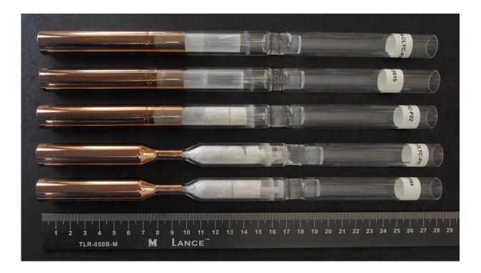
Flight ampoules for CLYC Crystal Growth samples, to be transported to the International Space Station. Resulting crystals will be compared against onground samples to develop on-Earth techniques for crystal growth. Credit: Alexei Churilov
