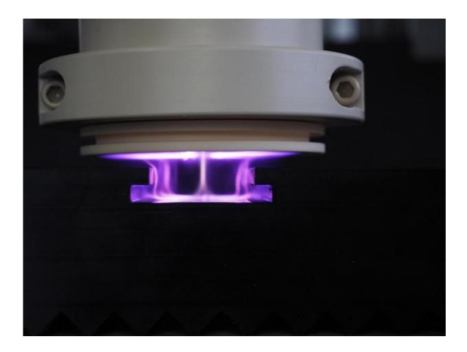
The Disc Jet can also be used to process cavities. Credit: HAWK
