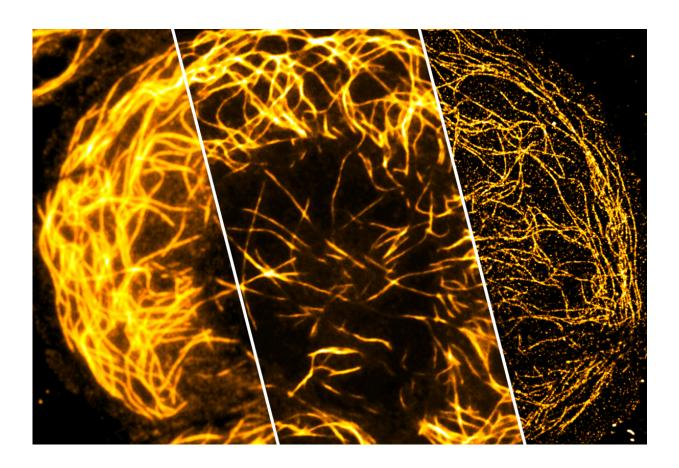
New imaging potential: Standard resolution (left) compared to (center, right) high resolution and super-resolution obtained with the chip-based technique. Credit: Bielefeld University/Robin Diekmann
