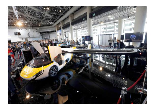
AeroMobil display their latest prototype of a flying car, in Monaco, Thursday, April 20, 2017. The light frame plane whose wings can fold back, like an insect is boosted by a rear propeller. The company says it is planning to accept first preorders for the vehicle as soon as later this year. (AP Photo/Claude Paris)
