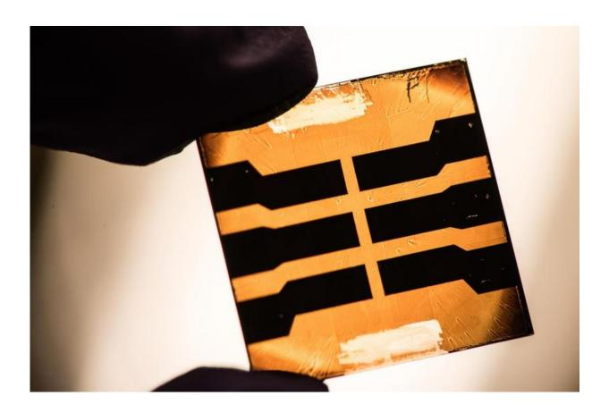
A lead sulfide quantum dot solar cell developed by researchers at NREL. Credit: Dennis Schroeder
