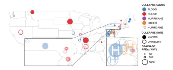
Of 35 bridge collapses analyzed, floods caused 13, erosion of sediments around bridge foundations -- scour -- caused 16, a hurricane caused 1 and other influences (such as waterborne or hydraulic debris) caused 5. Superimposed H denotes sites where a hurricane or tropical storm occurred and may have influenced bridge collapse. Area of circles is proportional to drainage area of bridge sites. Credit: Flint, et al.
