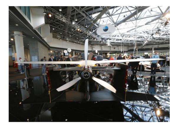
AeroMobil display a rear view of their latest prototype of a flying car, in Monaco, Thursday, April 20, 2017. The light frame plane whose wings can fold back, like an insect is boosted by a rear propeller. The company says it is planning to accept first preorders for the vehicle as soon as later this year. (AP Photo/Claude Paris)
