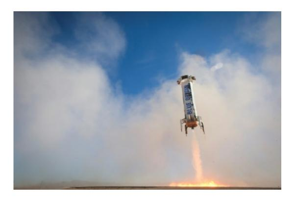
In this handout photo from Blue Origin, the rocket prepared for its third successful vertical landing in a test last year
