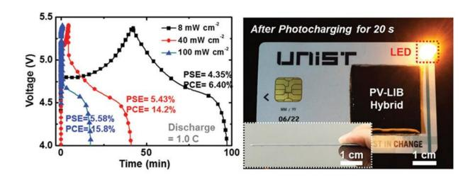
The SiPV-LIB device was fully charged under sunlight illumination after only 2 min and also even at a dimly-lit living room. The image on the right shows the operation of the SiPV-LIB-embedded smartcard. Credit: UNIST
