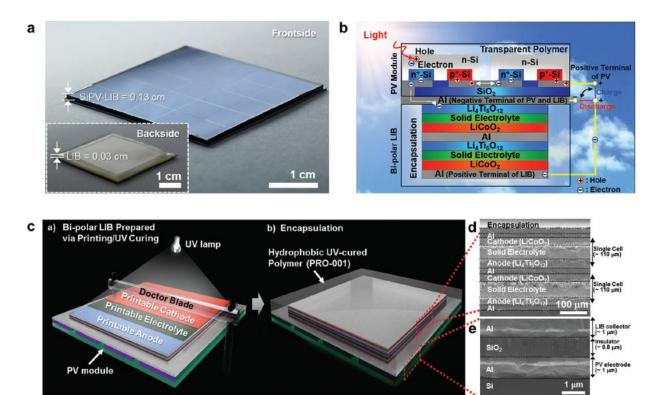
A schematic representation of the monolithically integrated SiPV-LIB device and the electrochemical performance of the bipolar LIB. Credit: UNIST
