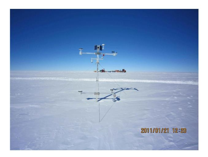
Automatic weather station on the Ross Ice Shelf, equipped with a Campbell Scientific SR50 acoustic depth gauge, which measures the distance to the snow surface from the speed of reflected sonic pulses. Credit: Minghu Ding
