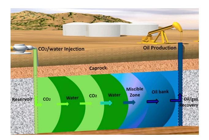
Schematic of the water-alternating-gas process for enhanced oil recovery. Credit: Los Alamos National Laboratory
