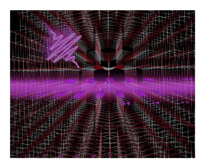
Lattice structure of anatase TiO2 with a graphical representation of the 2-D exciton that is generated by the absorption of light (purple wavy arrow). This 2-D exciton is the lowest energy excitation of the material. Credit: Majed Chergui/EPFL
