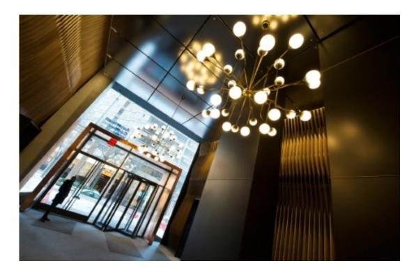
Planned just after deadly Hurricane Sandy hit New York, the lobby of the American Copper Buildings has open-sided wood panelling that dries easily with no damage in the event of flooding
