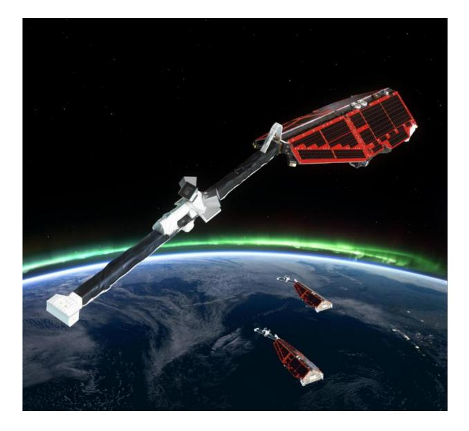
Swarm is ESA's first constellation of Earth observation satellites designed to measure the magnetic signals from Earth's core, mantle, crust, oceans, ionosphere and magnetosphere, providing data that will allow scientists to study the complexities of our protective magnetic field. Credit: ESA/AOES Medialab
