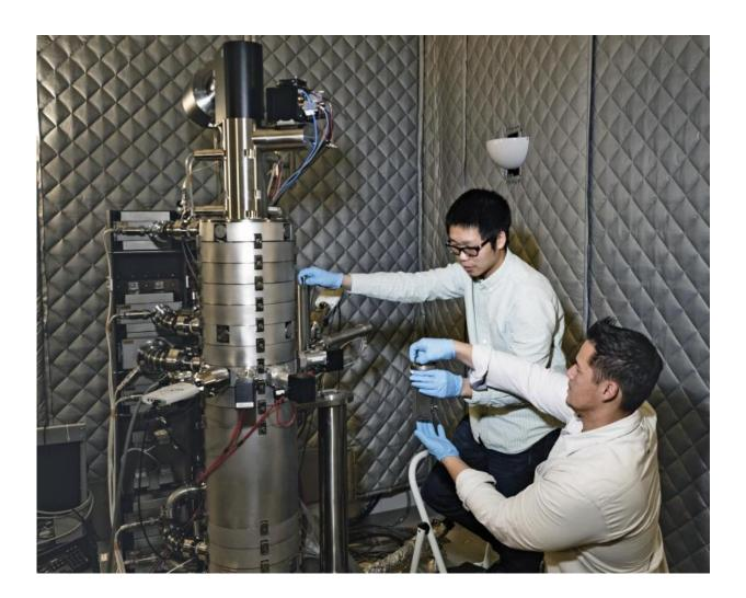
Xiahan Sang (left) and Raymond Unocic of Oak Ridge National Laboratory used scanning transmission electron microscopy and electron energy loss spectroscopy to reveal atomic positions and local electronic properties of 2D MXene that had been etched and exfoliated from a 3D crystal. Credit: Oak Ridge National Laboratory, U.S. Dept. of Energy; photographer Carlos Jones
