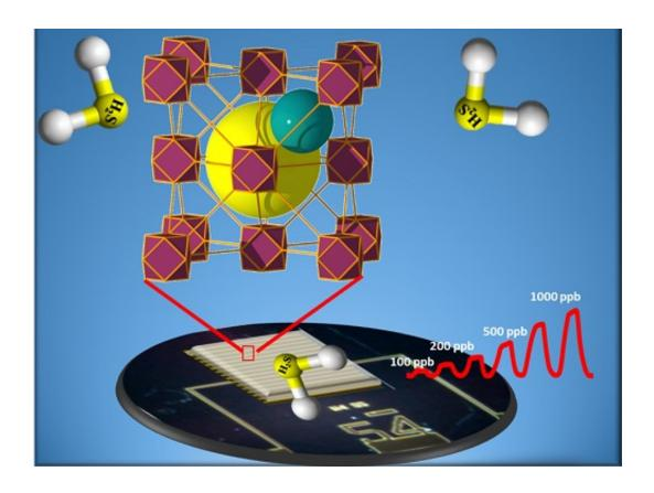
A carefully tuned MOF can detect the presence of hydrogen sulfide gas with ppb sensitivity. Credit: KAUST King Abdullah University of Science and Technology
